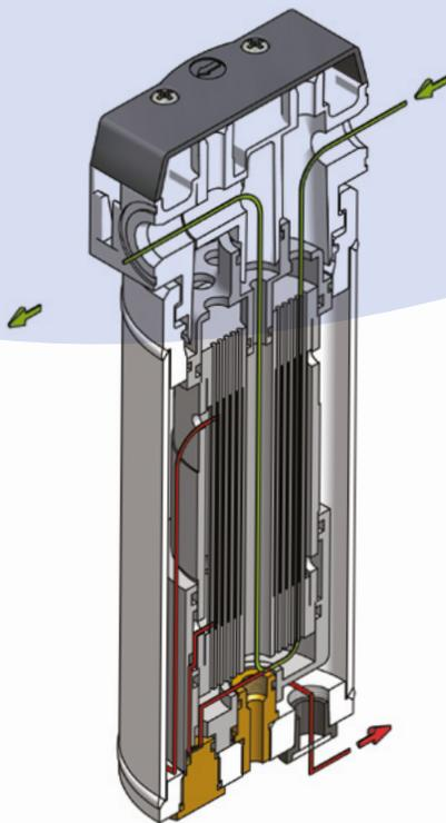
Pressure dew points from +50°F to -40°F are achieved by balancing the model size, air pressure and volume (scfm) requirements to the application.
