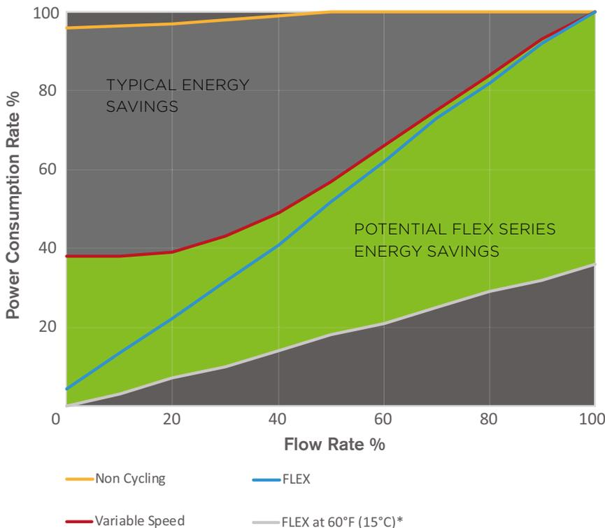
Dryers are rated in accordance to ISO 7183 standard rating conditions A2. (38°C / 100°F ambient)
